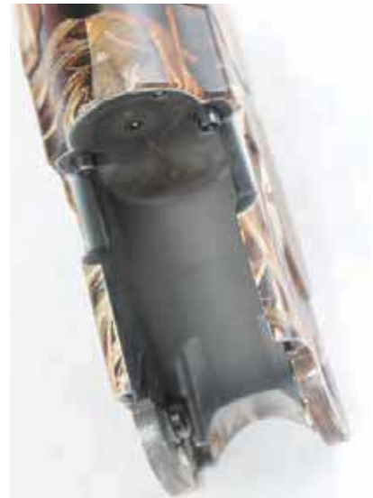
The protruding conical lugs from the top lock the gun and the barrels rotate on rounded replaceable trunnions located in the receiver walls, giving a low profile and nice balance.
