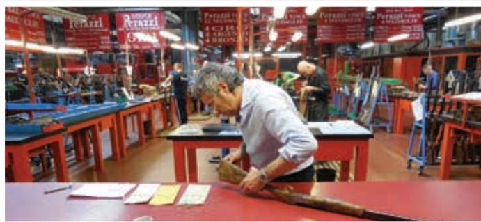
*Mauro carefully checking the stock's measurements after a test firing. Many guns are on the racks.*
